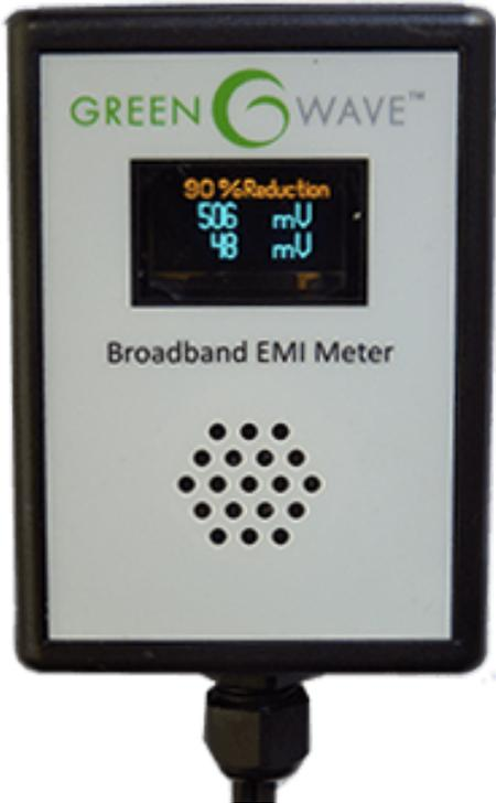
The *Greenwave® Broadband EMI Meter* is a revolutionary device for accurately measuring the level of dirty electricity (a.k.a., electrical noise, line noise, power line EMI) present on the wiring in buildings.
